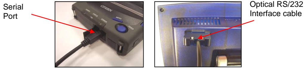
Figure 4.8: Connecting the printer to the Rapid 2 system
