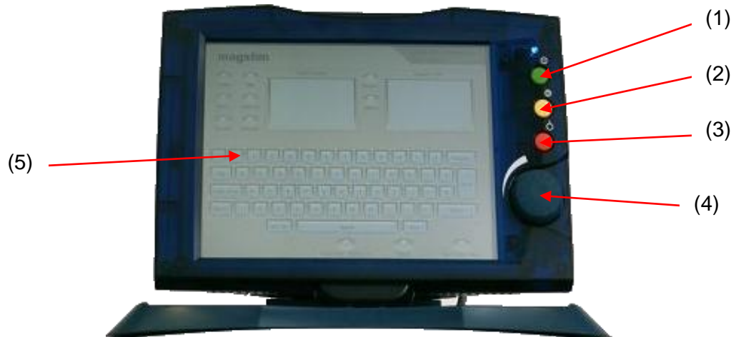
Figure 3.9: Detailed front panel of Rapid 2 UI.
