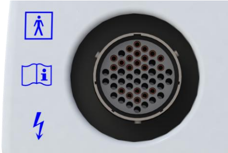
Figure 3.2: Coil output socket front view
